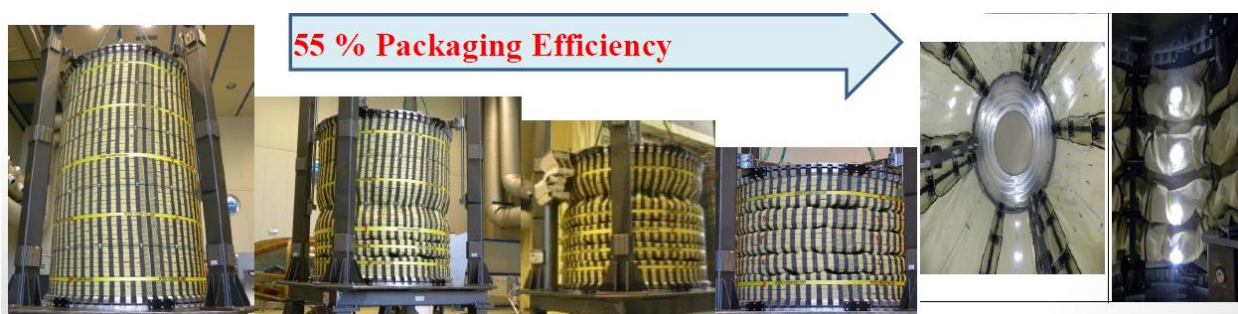
Figure 12-3: Full size crew lock foldable structure for ISS, with high packing efficiency and embedded sensor network RD[65]
