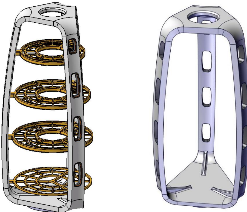
Figure 5-8: The main load-carrying structure
