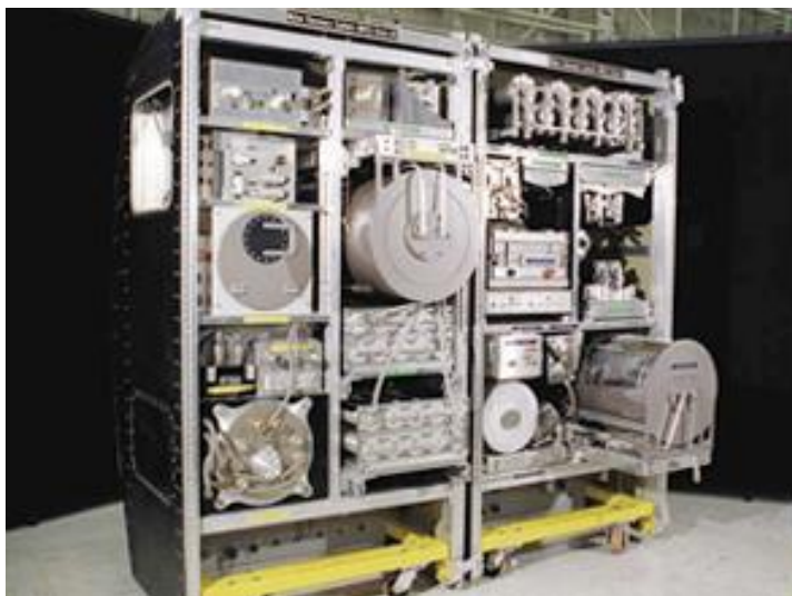
Figure 11-4: The ISS Water Recycling System, including the Urine Processing Assembly, the Water Processing Assembly and the Potable Water Dispenser
