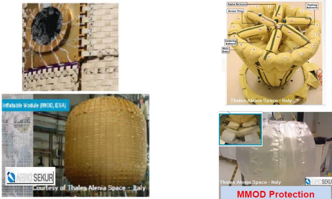
Figure 12-2: Inflation module demonstrator (left); inflatable docking mechanism (upper right); flexible expandable module with foldable micrometeoroid and debris protection (MMOD, lower right)[RD[65]
