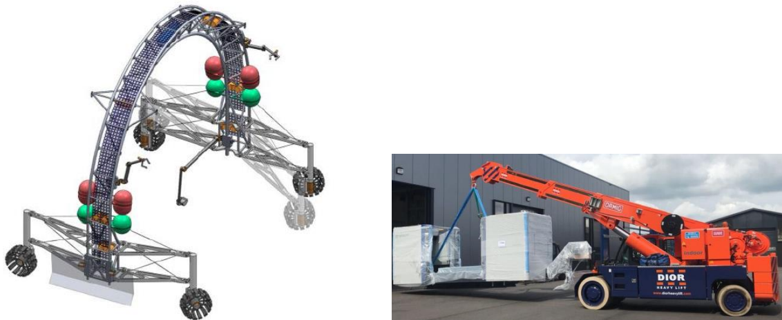
Figure 6-4: Mobile gantry crane (left) and pick-and-carry crane (right)
