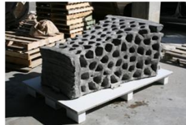
Large demonstrator 3D printed using regolith simulant
